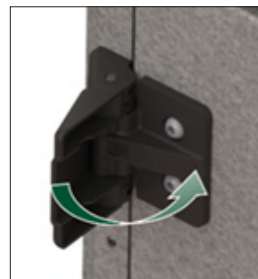
Pressure-relieving hinges; designed to avoid shearing damage to the service door gasket
